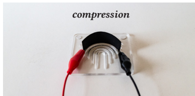
Experiment set-up: laser cut jig, alligator clip connections.
