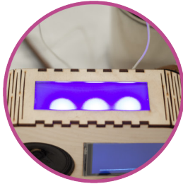
LED panel with pulsating light in shifting colors based on data
