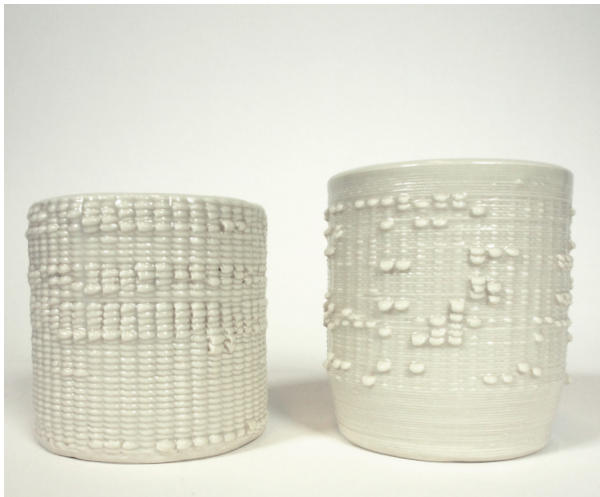
The size of the nozzle influenced the baseline thickness of the extruded clay. The left cup was created with a nozzle of 3.5 mm (and a layer height of 1.5mm) while the right cup was created with a nozzle of 2mm (and a layer height of 1.1 mm).
