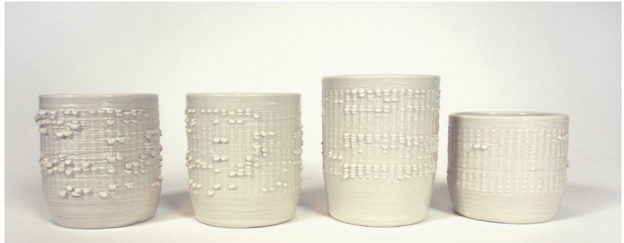
The longer the pauses, the more pronounced were the bumps. From left to right, we see how long pauses generate a coarse aggressive texture while shorter pauses yield a more delicate texture, almost reminiscent of weaving.
