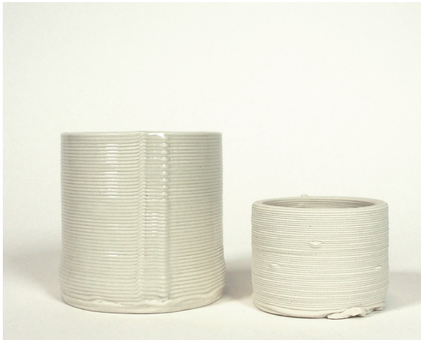
Early experimentations to see the impact of a bump amongst many lines (cup on the right) and the effect of repeating bumps at every line or every other line (cup on the left).
